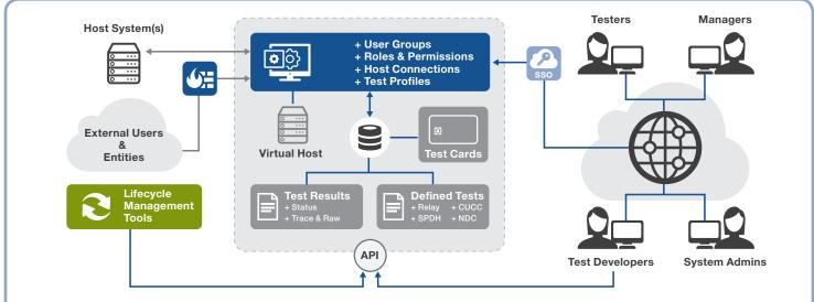
Web FASTest is a single platform to meet your payment testing needs: providing global access; supporting collaboration between multiple users at multiple sites; centralizing administration of user roles, permissions, and data; and enabling automation and integration.
