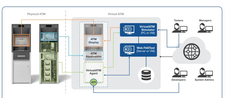
By virtualizing your existing ATM software stack and simulating its hardware, Paragon VirtualATM allows you to test your ATMs from anywhere. Testers can share media, run automated regression tests and integrate with other systems to help keep your virtualized ATM lab running smoothly.
